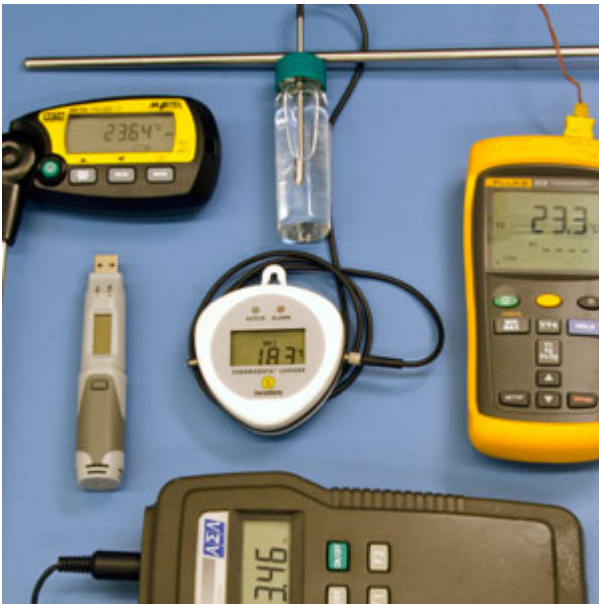
Temperature measuring devices (source: U.S. government)
